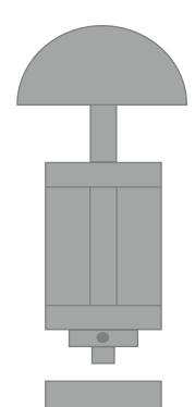
Slide bearing shaft into sleeve. Stop when the top bearing is flush with top of sleeve.
